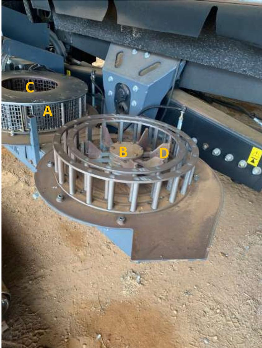
The Multi-Stage Hammer Mill is composed of both stationary and rotating component groups. Stationary (A) being the screen set, which is attached to the main chassis and Rotating (B) being the flails and rotor, which is attached to the hub/spindle assemblies.
