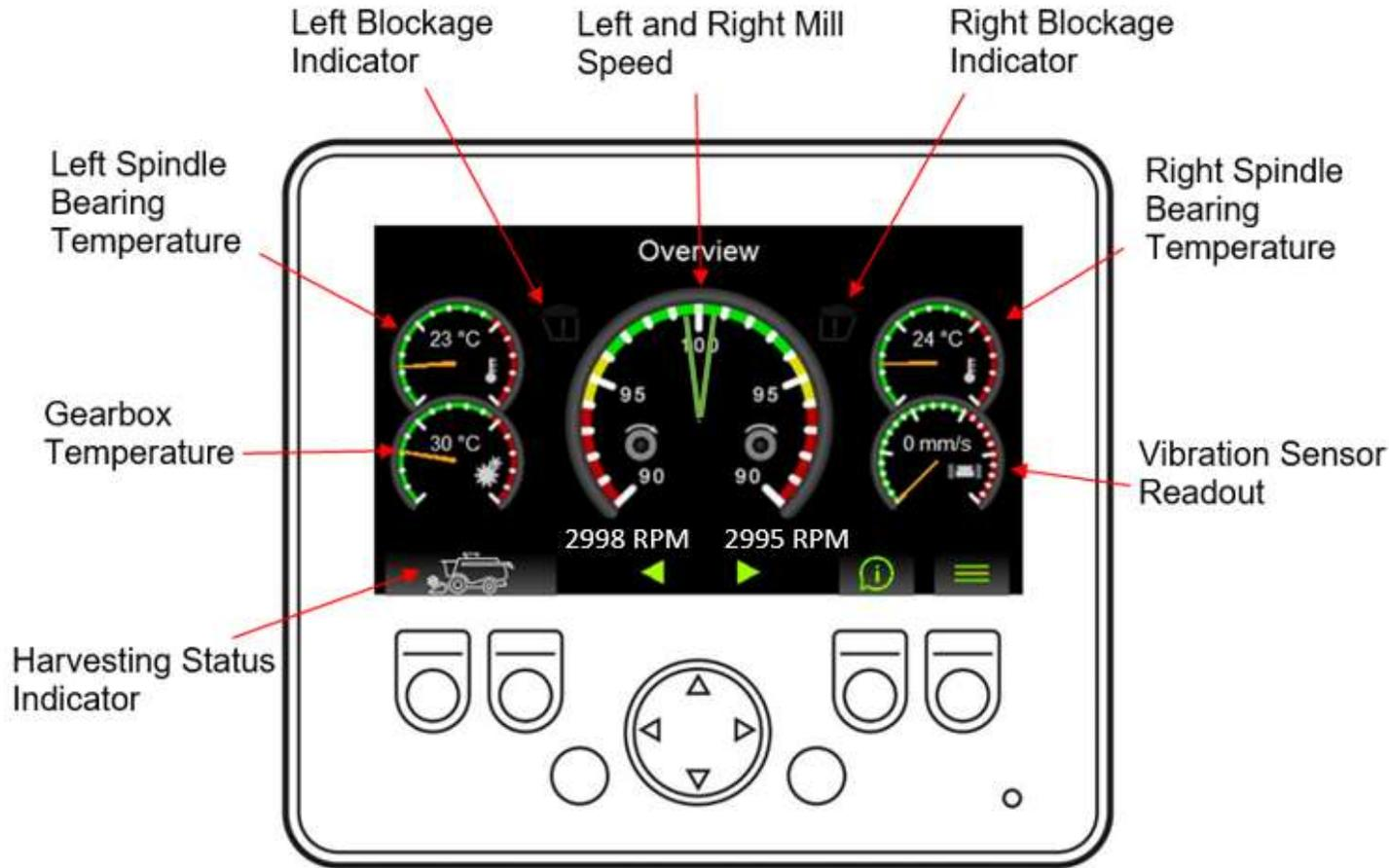
The Monitoring System consists of two main operational components and eight sensors. Both main components contain the programs to allow the system to operate. See below for a brief description.
